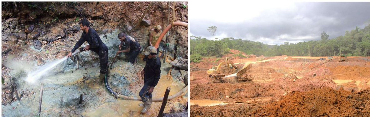
Figure 1.2. Illegal gold miners using a high-pressure water hose (left), and modern alluvial gold exploitation showing an excavator, gravel pump, screen with bars and gold mat. Reproduced from (Jébrak et al. 2021) with permission from P. Rostan.
